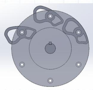
Added weight: weight is added in order to ensure that the dogs stays at its intended position
